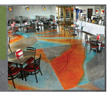
Brickform's® suite of decorative stains provide permanent, long lasting color to concrete surfaces. Both the ARTesian™ water-based stain and E-Stain™ reactive stain, prevent exposure to Volatile Organic Compounds or VOCs.
